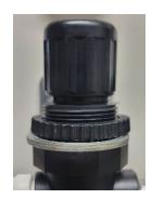
(The nozzle must be operating to perform this task). If drain flow is too much, turn the adjustment knob slightly counterclockwise to reduce flow to a steady drip. If needed, temporarily adjust the RH setpoint higher; this will turn the system on. Adjust back to desired RH when finished.
