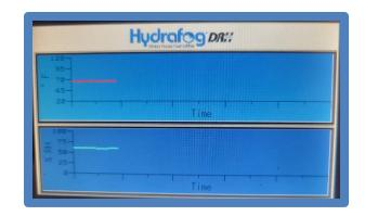
If you want to store your temperature and % relative humidity data into .csv spreadsheet files, insert a USB drive into the port located on the bottom of the HMI. Your data will be logged on 5-minute intervals. The USB directory is HGDATA01\DATALOG. The data is stored in daily files with the filenames:
