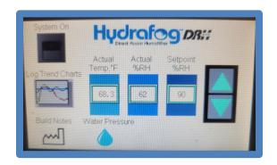
To turn on the HydraFog DRH system tap the "System On" icon. The green indicator light will indicate the system is ready to control the room's humidity.
