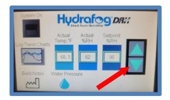
Tapping the arrow icons will bring up a protective passcode screen. The default programmed passcode for all HydraFog DRH systems is 1234. Pressing 1234 and then ENT will allow you to change the relative humidity setpoint with the arrows.
